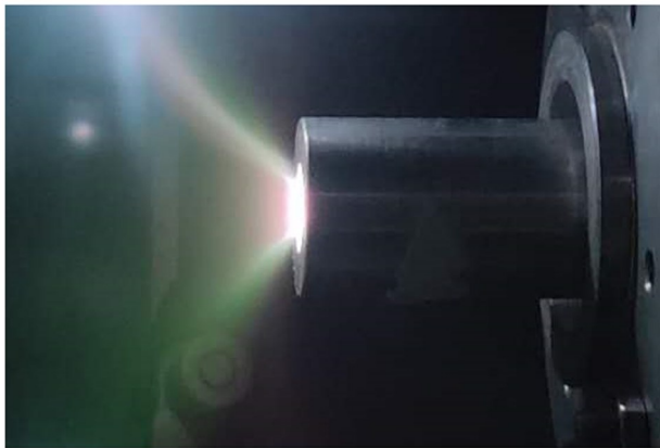
图 15 (a) 直流型会切磁场型霍尔推力器, (b) 推力调节范围 Fig. 15 (a) DC type Cusped field thruster, (b) thrust adjustment range
